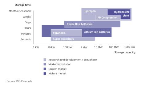
Storage techniques based on storage duration and storage capacity
