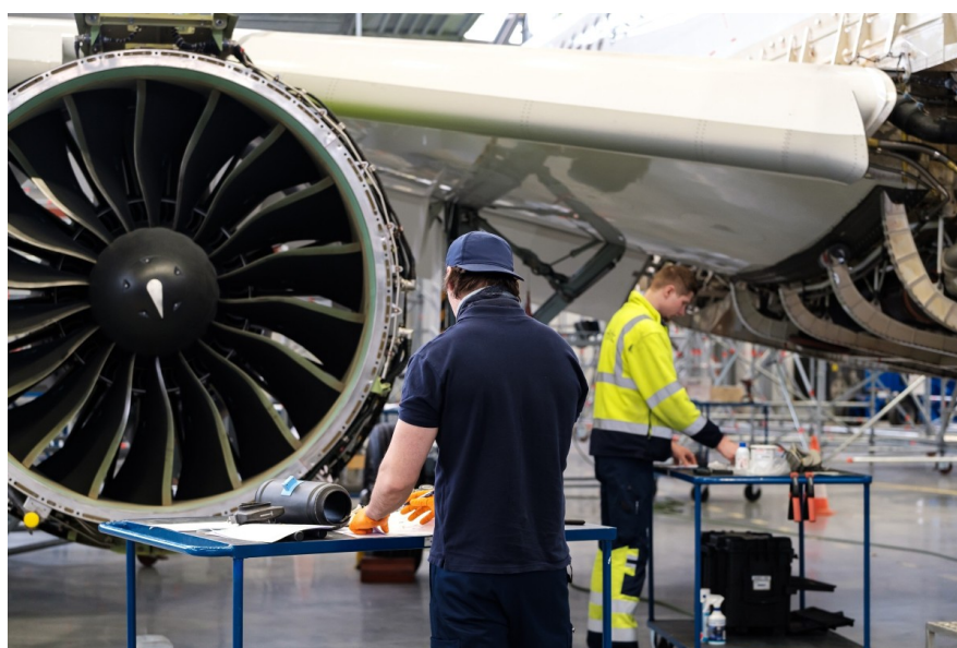
A partially disassembled Pratt Whitney PW1500G engine of the Airbaltic Airbus A220 aircraft
