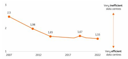
Source: Uptime Institute; A PUE of 2 means that for every watt of IT power, another watt is consumed for cooling and other non-IT equipment. A PUE of 1.0 means that all energy is used for computing.
