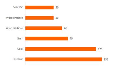
\*Combined Cycle Gas Turbines or CCGT power plants. The LCOE for gas peaker plants is much higher.
