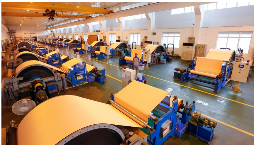
Workers on a copper foil production line in Jiangxi Province
