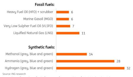
\*Number of yearly refuels for our reference ship of 82.000 deadweight tonnage with 230 sailing days per year at an average speed of 17 knots. The benchmark ship runs on HFO and needs to refuel 6 times a year given its tank size. We have calculated the amount of refuels for this tank size for every fuel type. The tank size holds less energy if it is filled with synthetic fuels and therefore needs to refuel more often. Note that all synthetic fuels are liquified.
