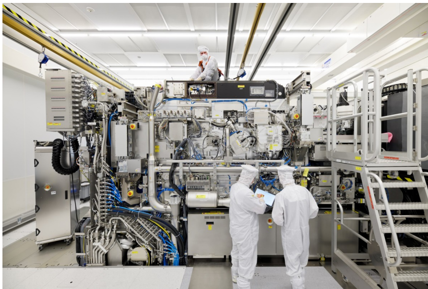
An ASML 'cleanroom' - an ultraclean environment where the company assembles EUV and DUV lithography systems
