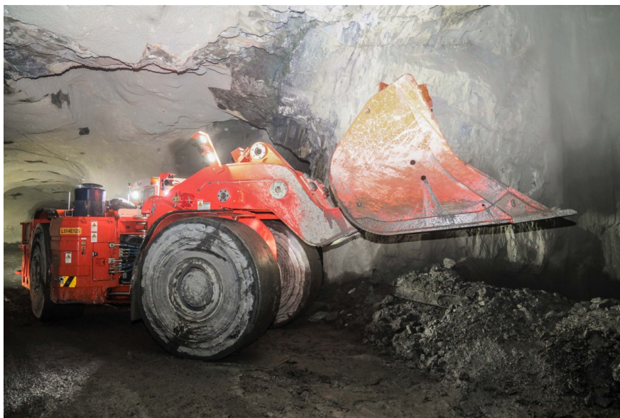
A remote-controlled shovel loader works underground at an iron mine in northeast China's Liaoning Province
