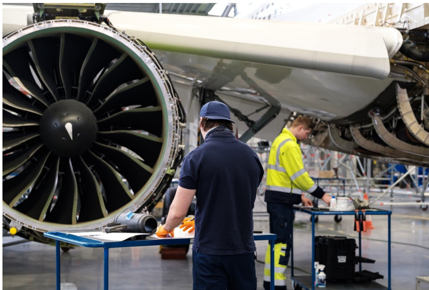
A partially disassembled Pratt Whitney PW1500G engine of the Airbus A220 aircraft
