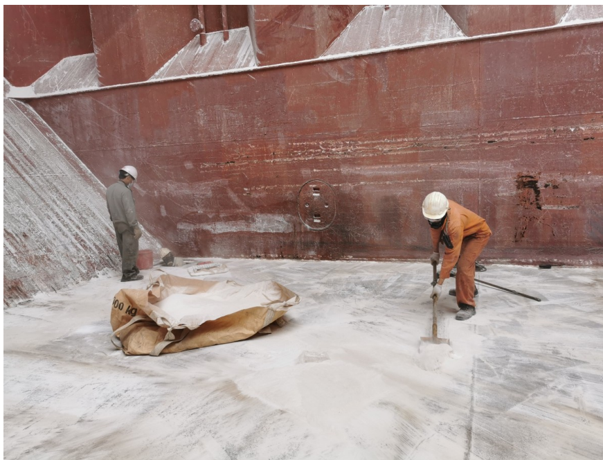
Ship crew sweeping alumina cargo residue in hold of a bulk carrier
